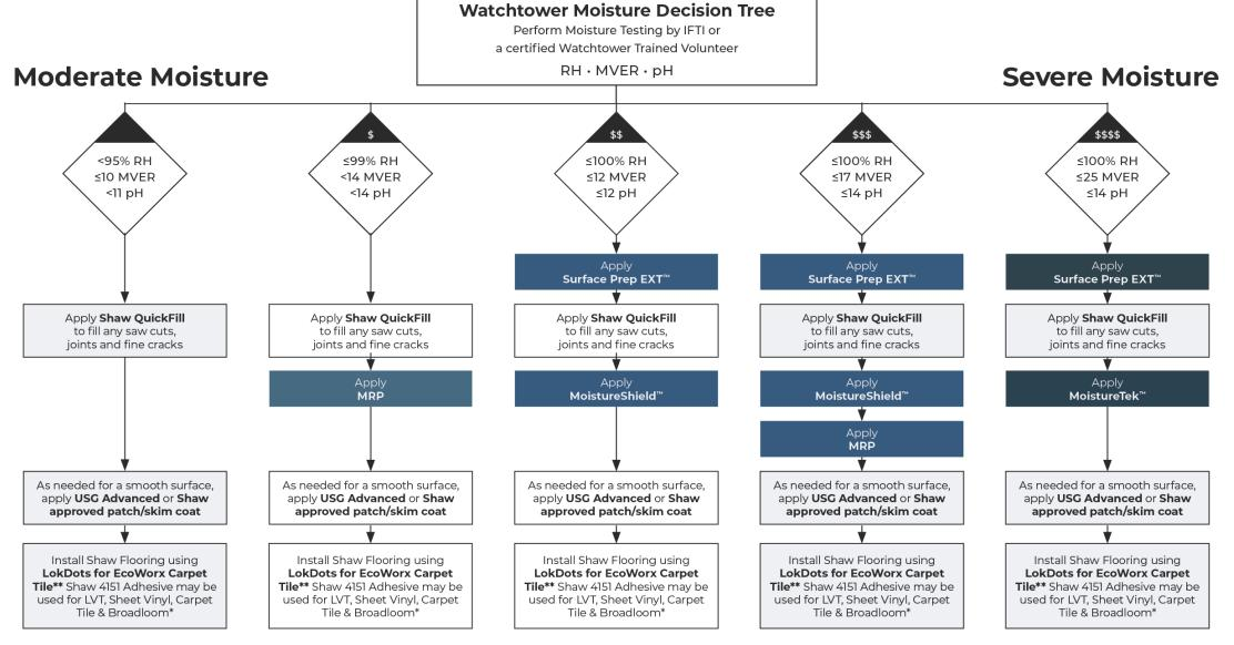
MVER - Moisture Vapor Emission Rate, measured by the Calcium Chloride Test
